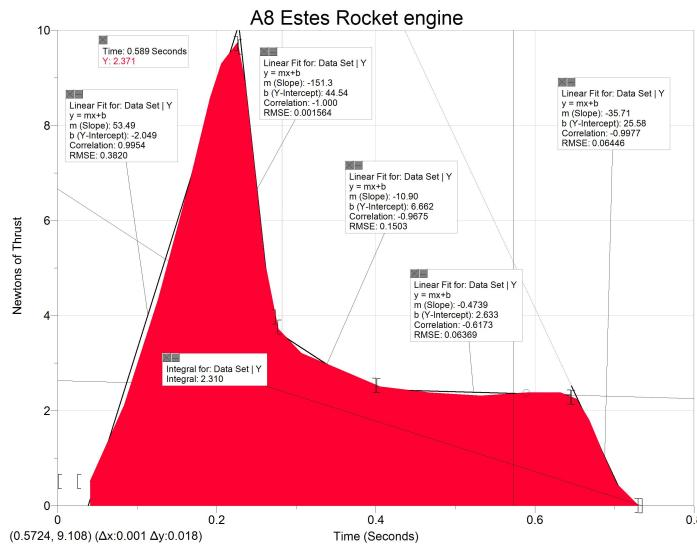
The following code displays a graph of the integral of the thrust force and time for the rocket motor which is known as the rocket motor's IMPULSE. The data used to determine the slopes of the thrust curve was experimentally determined using a Vernier Force Probe and a LabPro interface. The data was then put into this LB program and produced the image you see when the program was run.
